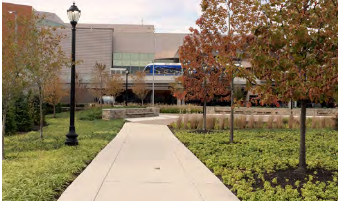
15'-20' wide promenade with saw cut concrete paving
